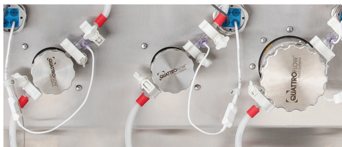
Figure 5. Three positive displacement pumps.
