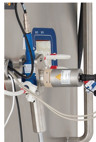
Figure 7. Post-column sensor pack with UV detector.
